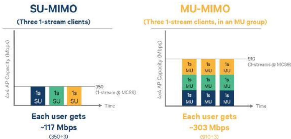
Figure 2-6 Throughput difference between SU-MIMO and MU-MIMO
